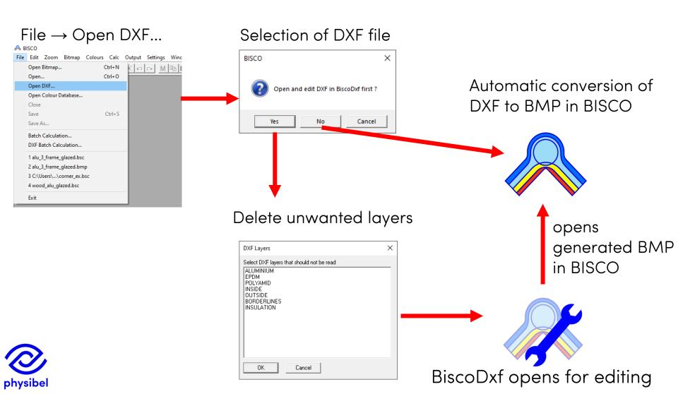
In BISCO v11 problems may occur when the 2D DXF files are extracted from 3D DXF files because of differences in extrusion direction
