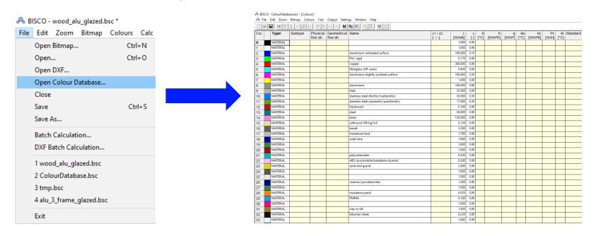
The default Colour Database delivered with the software is updated for EN ISO 10077-2, EN ISO 10456 and EN ISO 6946
