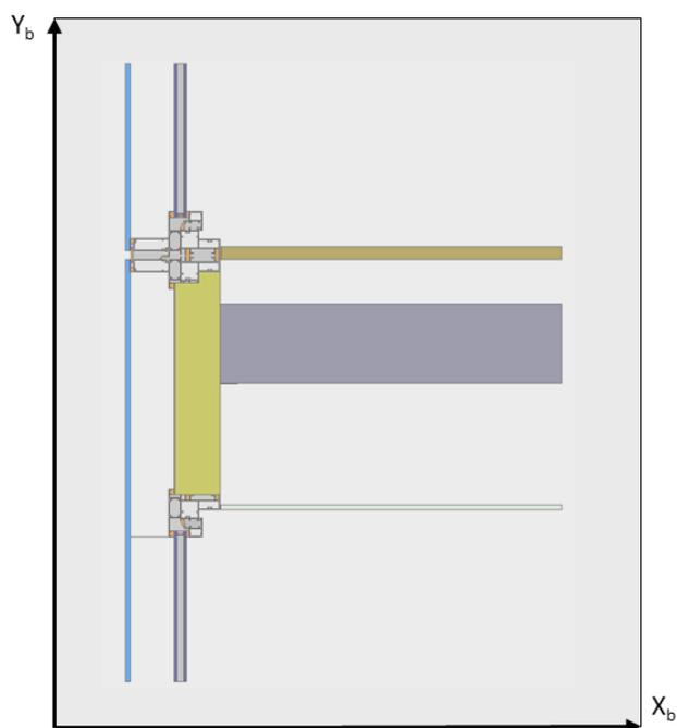
Since this is a vertical section, the first rotation angle equals  $0^\circ$  and the second rotation angle equals  $90^\circ$ . The third rotation angle thus determines the azimuth of the model. When the 3<sup>rd</sup> angle equals  $0^\circ$ , the bitmap positive X-axis points north, so the façade faces south. When the 3<sup>rd</sup> angle equals  $270^\circ$ , the clockwise angle between the bitmap positive X-axis and the north is  $270^\circ$ , so the façade faces west.
