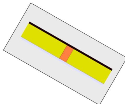
After the first rotation, the model can be viewed as a vertical section and the second rotation angle thus equals  $90^\circ$ . The third rotation angle determines the azimuth of the model. When the 3<sup>rd</sup> angle equals  $0^\circ$ , the bitmap positive X-axis points north, so the roof faces north.
