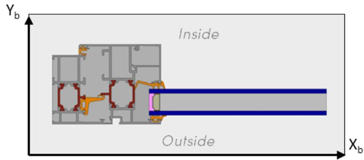
Since this is a horizontal section, the first rotation and second rotation angles both equal  $0^\circ$ . The third rotation angle thus determines the azimuth of the model. When the 3<sup>rd</sup> angle equals  $0^\circ$ , the bitmap positive X-axis points north, so the window faces east. When the 3<sup>rd</sup> angle equals  $270^\circ$ , the clockwise angle between the bitmap positive X-axis and the north is  $270^\circ$ , so the window faces south.
